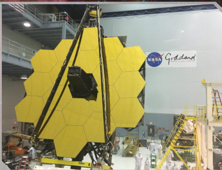
Main mirror of the James Webb Space Telescope assembled at Goddard Space Flight Center, May 2016. 8
